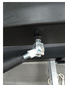
Fixing of the tie rod plates
